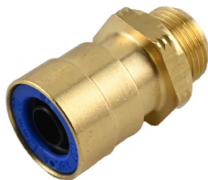
A.B.C PUSH-IN - STRAIGHT 12MM - 3/8 NPT
